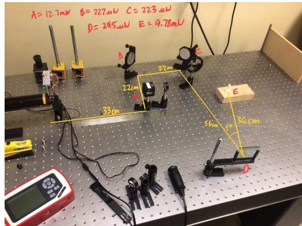
Figure 5: The Fourier Hologram Setup
