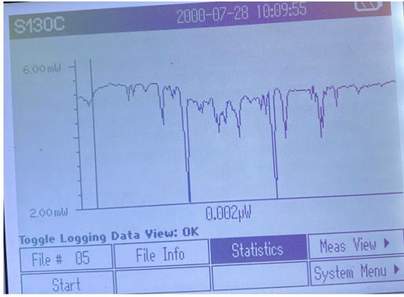
Figure 8: Intensity as a function of time, total time was 1 minute 23 seconds
