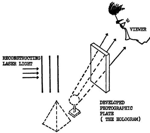
Figure 2: Viewing a hologram [1]
