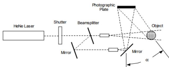
Figure 3: Fourier Transformation hologram optical setup [2]
