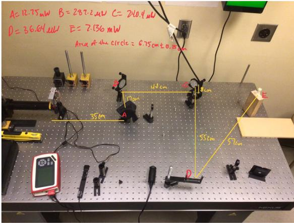
Figure 6: We also tried a second Fourier arrangement. In this one the distance to the object is the same as the distance to the last mirror of the reference beam. This will be referred to as Fourier 2.
