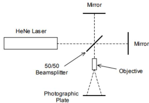
Figure 4: The Michelson interferometer [2]
