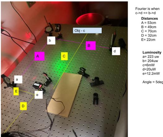
Figure 7: The Fresnel hologram setup
