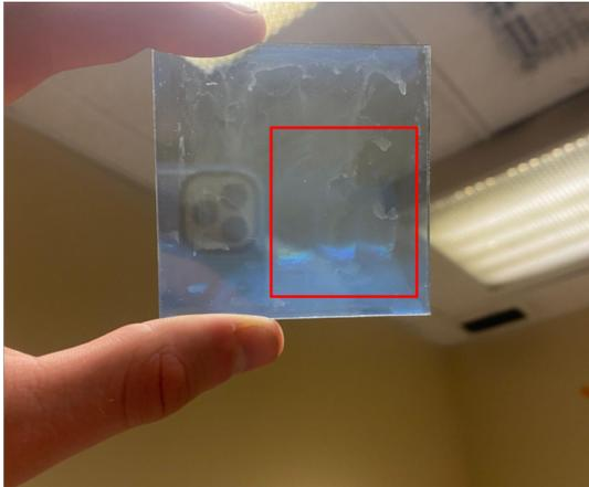
Figure 9: Three crests recorded onto a photoplate with different exposure times
