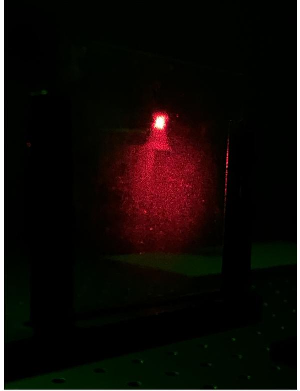
Figure 10: The first image from the Fresnal hologram, a fairly distinct virtual image around the location of the object
